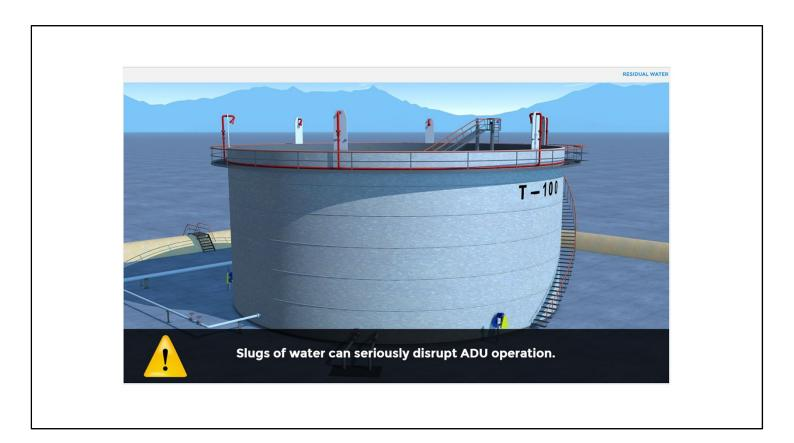
Before a crude can be run through the ADU, crude receiving tanks must stand for sufficient time to allow any residual water to disengage, accumulate and be drained off - slugs of water can seriously disrupt ADU operation.
