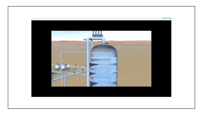
The ADU makes extensive use of distillation to separate crude oil into gas, light/middle/heavy distillate and residue products.
