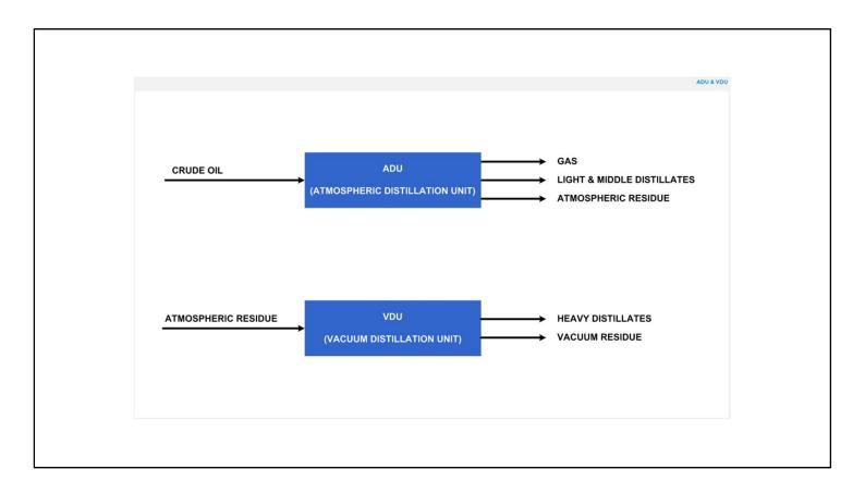
So, we know that an Atmospheric Distillation Unit (or ADU) separates crude oil into gas, light and middle distillate and atmospheric residue fractions.
