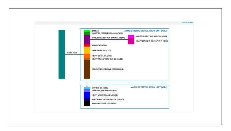
This diagram shows the VDU product streams - these are significant because HVGO, VHVGO and Vac Resid are used in ADU-VDU heat integration.
