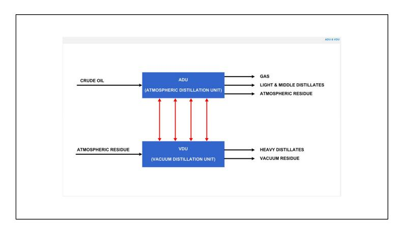
Although the ADU and VDU are separate process units, for the purpose of efficient utilization of energy their heat recovery systems are often integrated. Integration takes the form of indirect heat exchange between hot VDU pumparounds/products and cold ADU crude feed.
