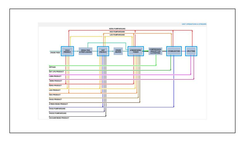
This diagram illustrates how the ADU feed, intermediate, product and pumparound streams together with the VDU product and pumparound streams are heat integrated with the Cold Preheat, Hot Preheat, Atmospheric Tower, Stabilization and Splitting unit operations. As you can see, its complex.
