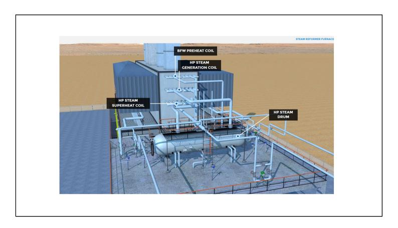
This image shows the High Pressure Steam Drum and its interconnecting pipework to the boiler feed water preheat, steam generation and steam superheat convection coils.
