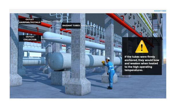
The outlet hairpins also facilitate expansion and contraction of the radiant tubes.
