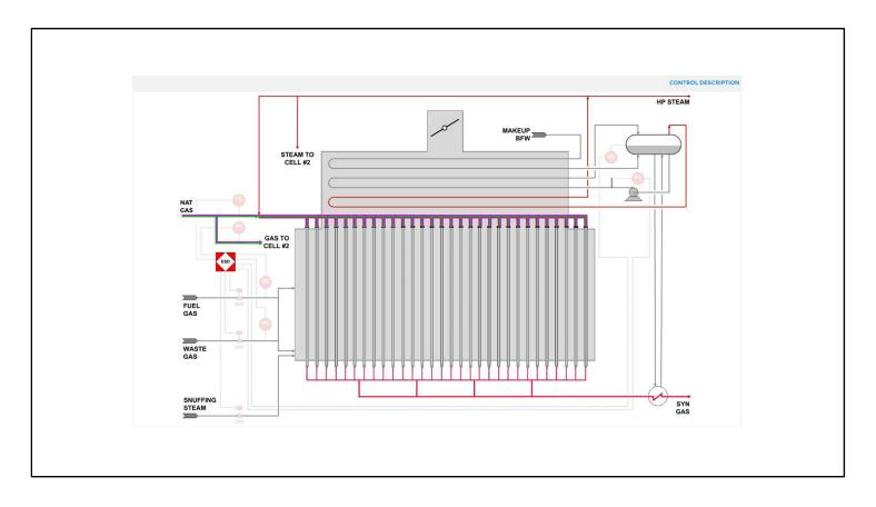
The Reformer Furnace and its catalyst are protected by an ESD system, which is activated by:
