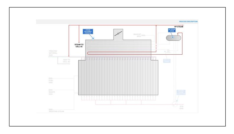
Makeup boiler feed water passes through a preheat coil in the convection section before entering the High Pressure Steam Drum.
