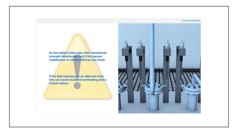
With careful operation, the reformer radiant tubes should achieve a life-time of around 100,000 hours (or 10 years).
