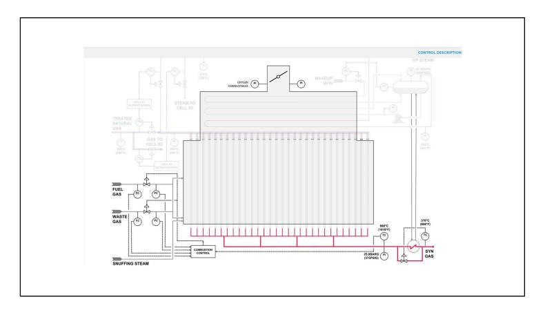
The combustion controller adjusts the refinery fuel gas and waste gas streams in a 30:70 ratio, with refinery fuel gas meeting the baseload.
