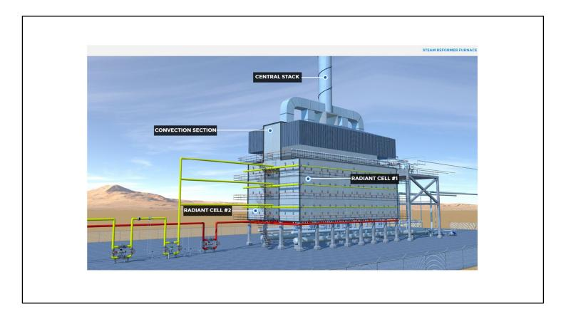
Steam-methane reforming is carried out in a Steam Reformer Furnace.
