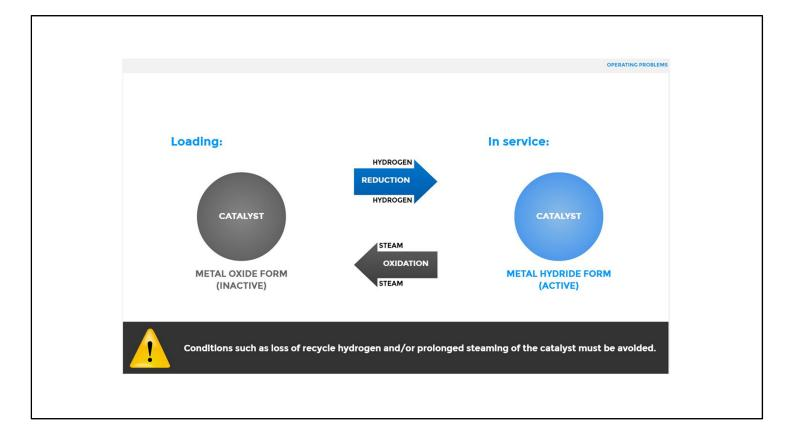
The radiant tube catalyst, as loaded, is usually in its metal oxide (inactive) form.
