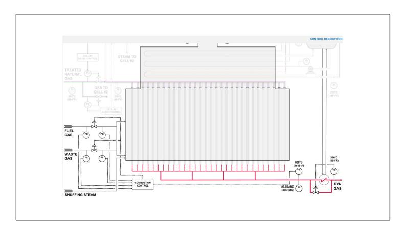
A combustion controller maintains the temperatures of the two outlet collectors at 880°C (1,616°F) - these two temperatures determine the extent of the reactions that take place in the radiant tubes.
