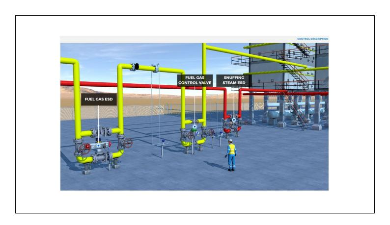
This image shows the primary fuel gas ESD and control valves and the snuffing steam ESD valve.
