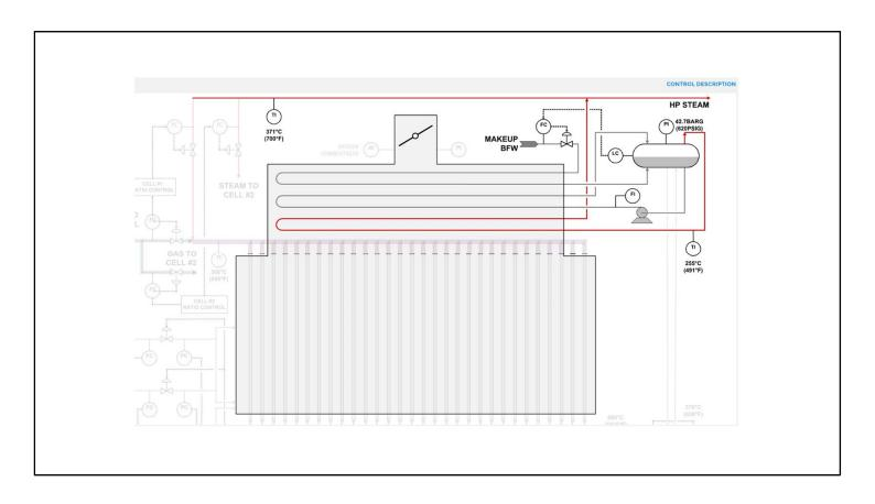
The High Pressure Steam Drum has a constant makeup of preheated boiler feed water, maintained by a level to flow cascade control arrangement.
