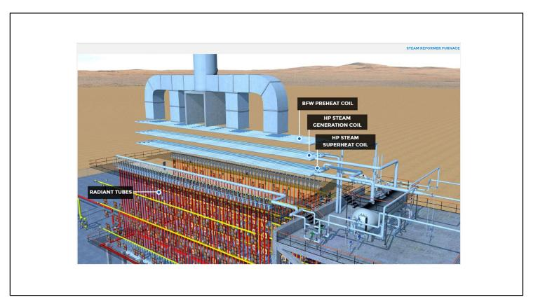
Each radiant cell has a central row of 48 tubes that are packed with catalyst, over which a mixture of steam and methane is passed and chemical reactions take place.
