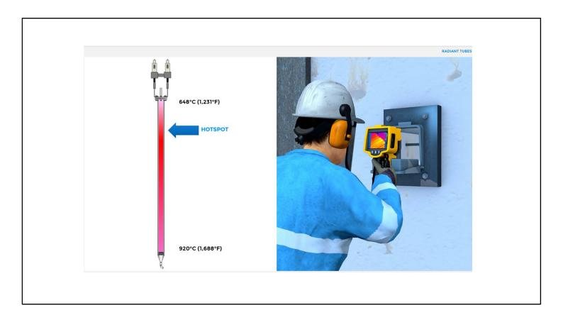
The radiant tubes are subject to a substantial temperature differential from top to bottom.
