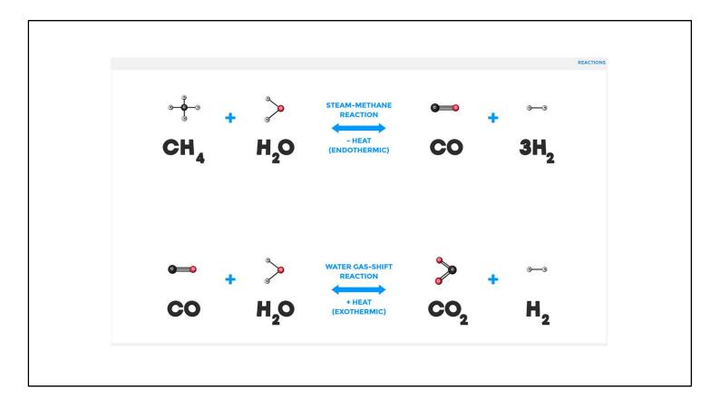
There are two reactions that take place as superheated steam and methane pass across the catalyst in the radiant tubes.
