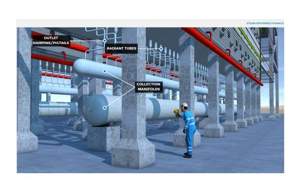
The outlets of the radiant tubes are connected via hairpins to two collection manifolds.
