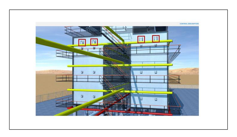
As additional protection against damage, the radiant cells have a number of hinged explosion doors that relieve pressure in the event of a firebox explosion.
