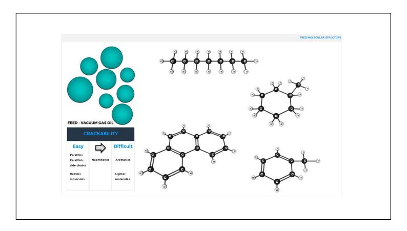
The VGO hydrocarbons are arranged in paraffinic, naphthenic, aromatic and poly nuclear aromatic structures.
