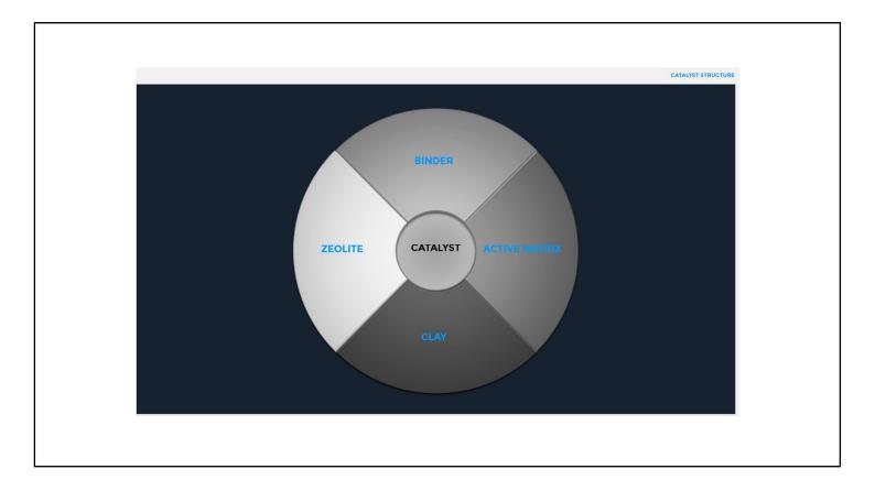
Let's take a brief look at the structure of the catalyst, which has four components - active matrix, zeolite, clay and a binder:
