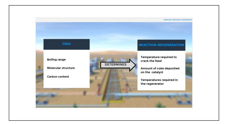
We'll finish up this module by pointing out the principal constraints on FCC operation – there are quite a few and they're going to surface in the following modules in the sections on operating problems. For now, we'll just consider the main two.
