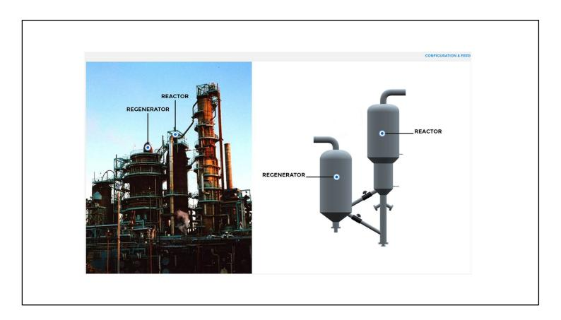
In this e-learning program, we're going to limit our discussions to a side-by-side reactor-regenerator configuration with a sweet (i.e. hydrotreated) VGO feed with no inclusion of heavier stock.
