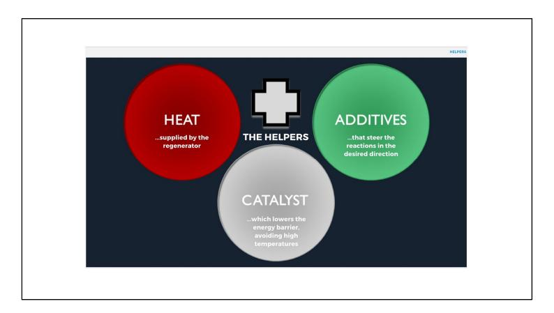
The endothermic cracking reactions are helped by heat (supplied by the regenerator), catalyst (which lowers the energy barrier, avoiding high temperatures that lead to undesirable thermal cracking) and additives (that steer the reactions in the desired direction).
