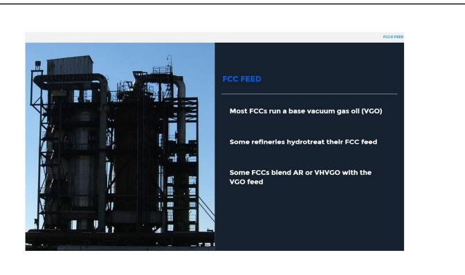
In addition to reactor-regenerator configuration, FCCs also have variations in the type of feed that is run.
