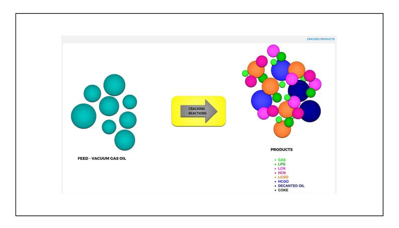
The reactions generate a number of cracked products such as gas, LPG, LCN, HCN and LCGO together with residues of HCGO and Decanted Oil, which are essentially the uncracked portion of the feed.
