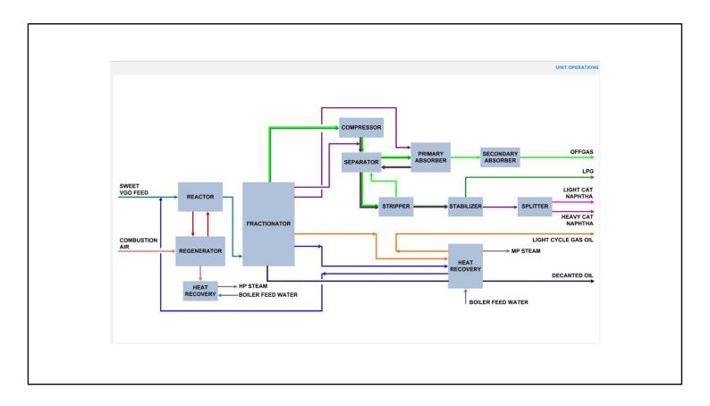
The FCCU has several unit operations that are split into modules as shown in this diagram:
