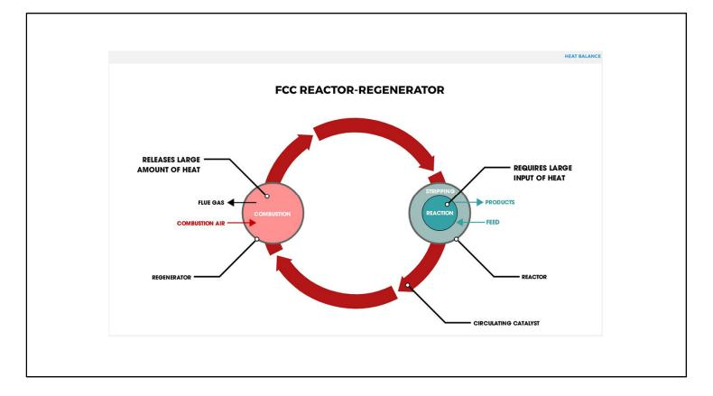
This simple diagram represents the reactor-regenerator system. Hot catalyst circulates continuously between the reactor (on the right) and the regenerator (on the left).
