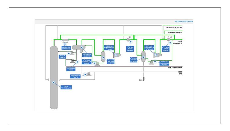
The purpose of the Gas Plant is to separate the Main Fractionator overheads and upper side draw into offgas, LPG and Light and Heavy Cat Naphtha.
