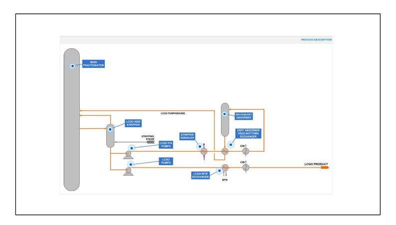
LCGO is withdrawn from the Main Fractionator as a mid side draw and passed to a Side Stripper where it is steam stripped to recover light hydrocarbons that are returned to the tower. From the bottom of the Side Stripper:
