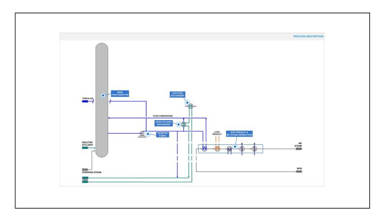
HCGO is withdrawn from the Main Fractionator as a lower side draw:
