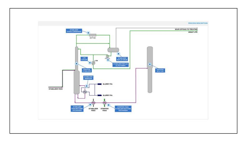
The Stabilizer feed enters the Stabilizer tower, where it is fractionated into:
