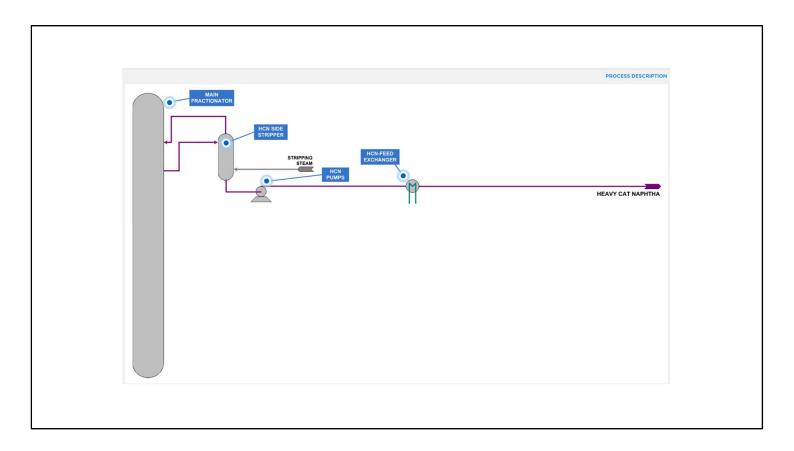
HCN is withdrawn from the Main Fractionator as an upper side draw and passed to a Side Stripper where it is steam stripped to recover light hydrocarbons that are returned to the tower.
