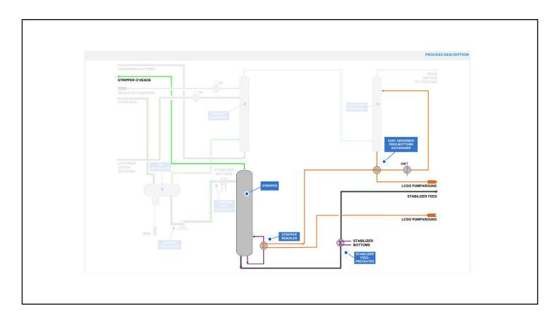
The Stripper, which is reboiled by LCGO pumparound, removes light gases such as methane, ethane and ethylene, which are withdrawn as an overheads stream and returned to the HP Separator via the Wet Gas Compressor 2<sup>nd</sup> Stage After Cooler.
