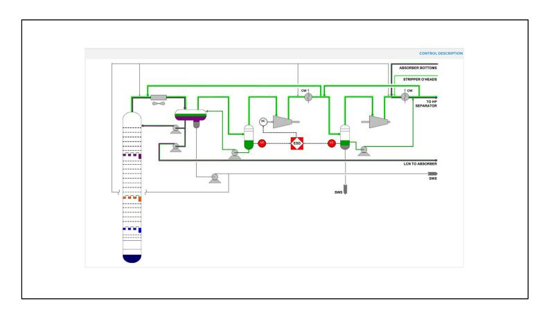
The Wet Gas Compressor is protected against mechanical damage due to the presence of liquid in the suction gas by an ESD system that trips the machine if there is a high level in either of the 1<sup>st</sup> or 2<sup>nd</sup> Stage KO Drums.
