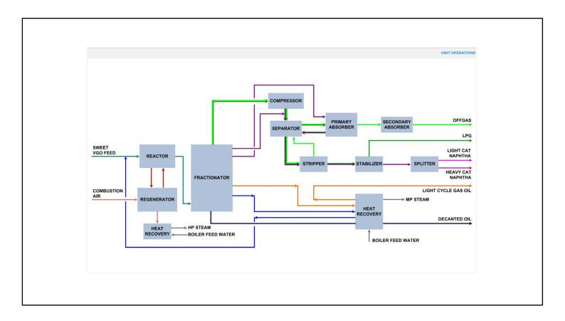
The Main Fractionator separates the Reactor effluent into overheads, side & bottoms products:
