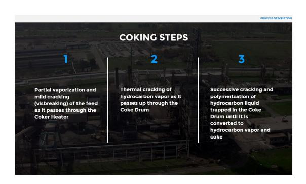
Delayed Coking is an endothermic process with the Coker Heater supplying the necessary heat of reaction.
