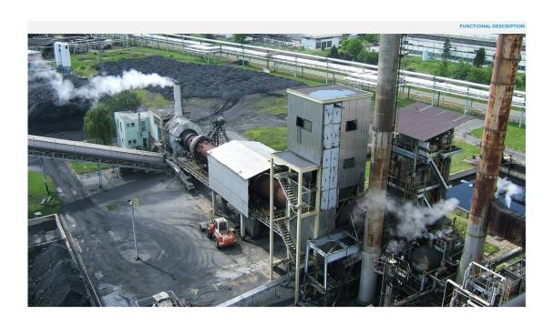
Further processing of green coke by calcining in a rotary kiln at 1,300°C (2,375°F) removes residual volatile hydrocarbons from the coke.
