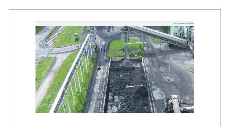
From the Cool Pit, green coke is transferred by conveyor to the Calciner.
