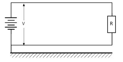
Network with one polarity grounded
