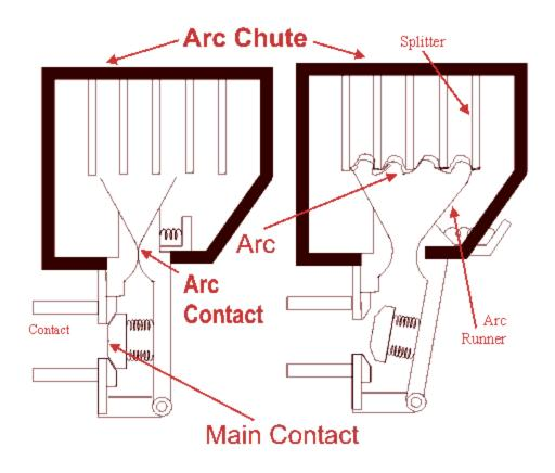
This kind of circuit breaker uses electromechanical contacts to achieve the required circuit isolation, while the electric arcs generated when the contacts open is used to help to dissipate energy stored in circuit inductance.
