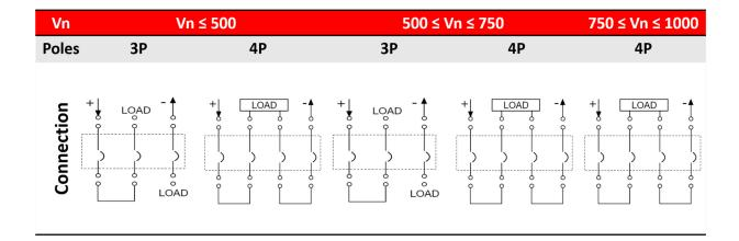
(i) The higher the number of poles opening the circuit, the higher is the breaking capacity of the circuit breaker.
