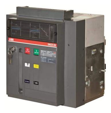
The ACB series Emax is divided into four basic sizes (E2, E3, E4 and E6) with an application field from 800A (with E2) to 5000A (with E6) and current breaking capacities ranging from 35 kA to 100 kA (at 500VDC).
