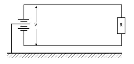
Network with the middle point of the supply source connected to ground
