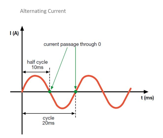
Interrupting a fault in AC is easier due to the nature of the alternating current. As the figure shows, the current in AC crosses through zero at each half cycle. Therefore, the electric arc which is formed during the current interruption process is extinguished naturally the moment in which the current returns to zero.
