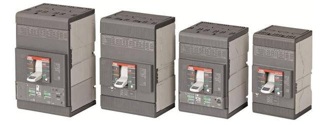
The molded case CB series SACE Tmax XT is divided into six basic sizes (XT1, XT2, XT3, XT4, XT5 and XT6), with an application field from 1.6A to 800A and current breaking capacities ranging from 16 kA to 100 kA (at 250VDC with two poles in series).
